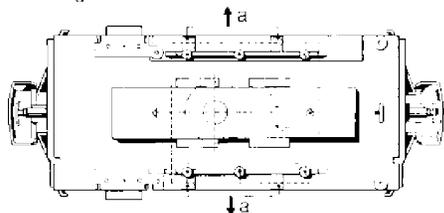
Loosen lead weight and gearbox cover in order to replace motor.
