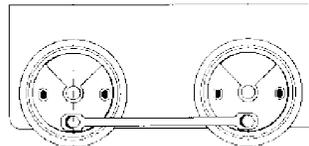
During assembly when the coupling rod is screwed into the pivot, it is vitally important to make sure that the coupling rod does not clamp at any wheel position. This would otherwise inevitably cause poor driving quality and may even destroy the gear.
