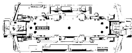
Remove gearbox base to replace contact shoes.
